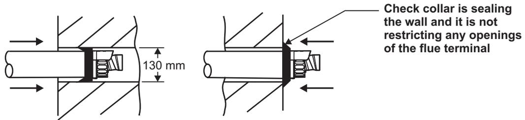
**Fig. 18 - Fitting the flue from inside**
