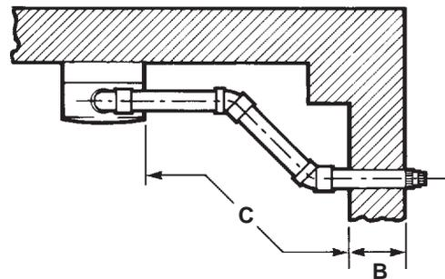
$$L = B + C + 245 \text{ mm} + (2 \times 45^\circ \text{ bends} = 1.8 \text{ metre})$$
