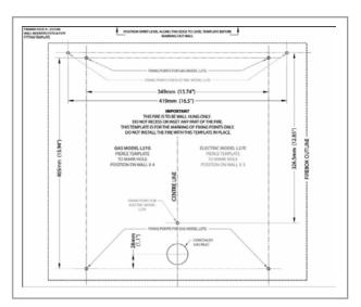
If the appliance is to be mounted on the inner leaf of a conventional cavity wall, or a solid wall, drill four holes to a depth of 42mm using a 8mm masonry bit. Insert the wallplugs provided.
