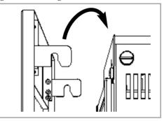
**L23 Chesire models and P23 Enigma models:** Remove the glass facia panel from any protective packaging. The glass facia panel is supported by four M6 screws which protrude from the front of the outer casing.
