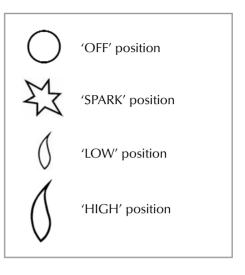
To turn to the PILOT position from the HIGH or LOW positions, press the control knob in, and return to the pilot position and release. To turn the fire OFF, keep the knob pressed in, return to the off position and release.
