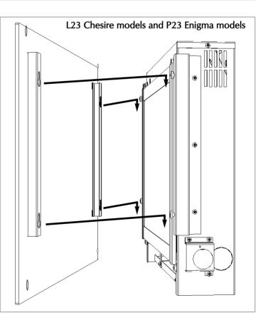
Compress the column assembly and position behind the glass panel, lining up with the appropriate hole. Release the assembly when in position and secure in place by refitting the front clamping disc.
